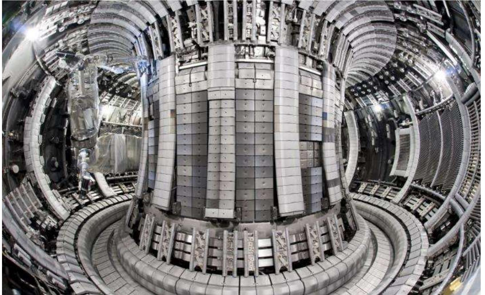
A Tokamak is a device which uses a magnetic field to confine plasma in the shape of a torus
